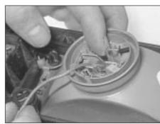
5.19 Releasing the auxiliary light bulb retainer (XR2i models)
